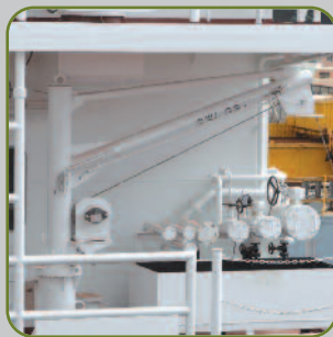
Fuel Oil Hose Handling Davit
